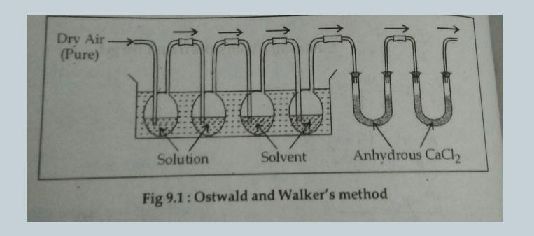
when air is passes through solution, it gets saturated with vapour. The vapours are carried forward and weight of solution bulb decreases.
